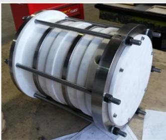
Active multi-effect distiller prototyped for energy-efficient desalination in remote areas. **SALTLESS project**
